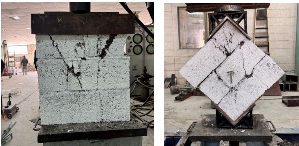
Figure 6: a) Prism compression test b) Diagonal compression test.
