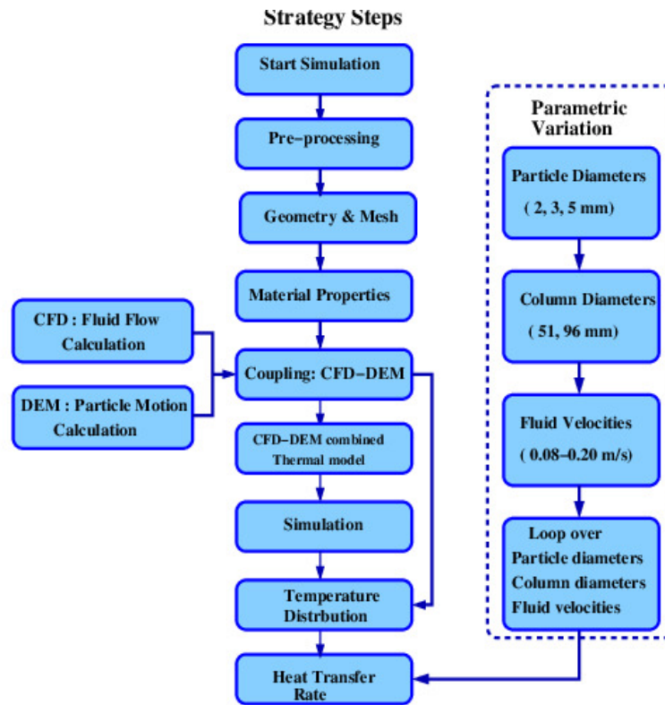
Figure1. Flow chart of the CFD-DEM approach to the simulation of heat transfer in a liquid-solid fluidized bed.
